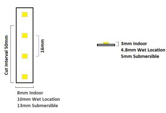
Specifications are typical values and may change without notification. Lumenova  $^{\text{TM}}$  and related graphics are trademarks of CRS Electronics, Inc.
